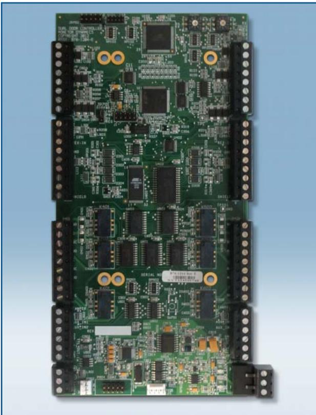
When a card's record is not found in the DDC database, the card data is passed to the NLC for the access control decision. If communication between the DDC and NLC is disrupted, the DDC continues to make access decisions for its 20,000 cardholders. Up to 512 events are stored at the DDC and passed to the NLC when communication is restored.
