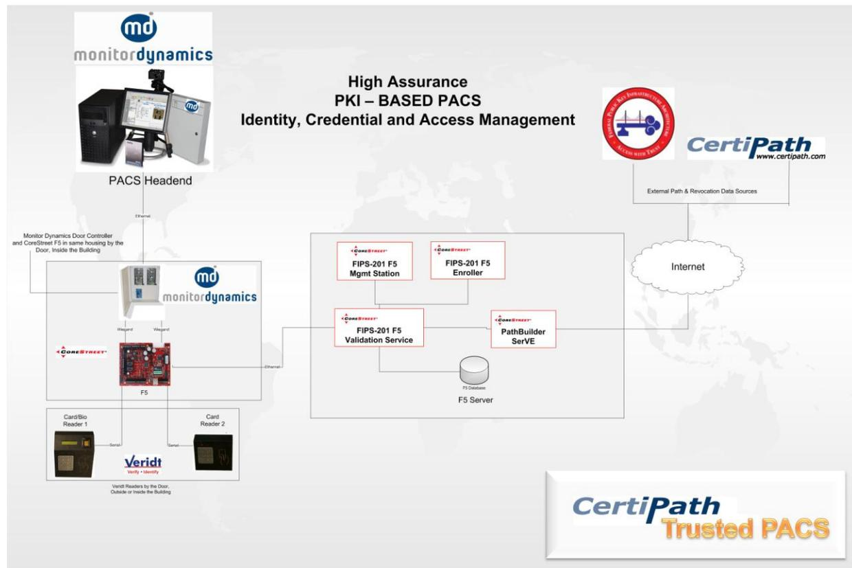
**Figure 1:** PIV Enabled PACS using the Panel Augmentation Approach
